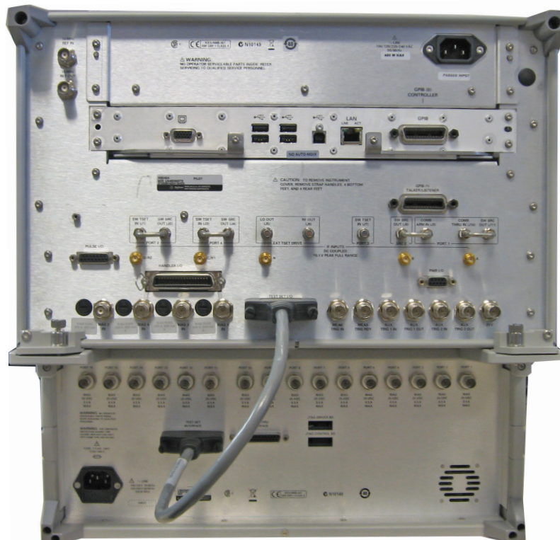
Figure 18 PNA-X Test Set I/O Cable Connection
